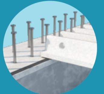
This sealant has been specially designed to stop ingress of water during the life of the structure and also to prevent any grout loss when pouring. It has been tested to prove excellent adhesion against two substrates, the maximum force required to remove the panel after sealing is equivalent to 6.15kN/m run of panels.
