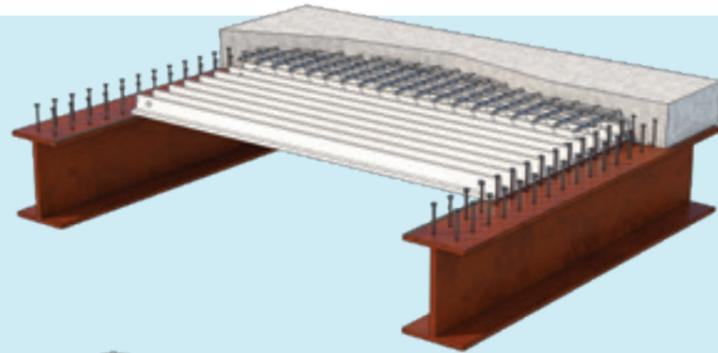
Typical EMJ Permadec Haunched panel installed on steel beams
