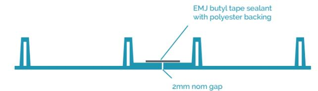
EMJ Butyl 2 x 6mm Ø Twin-track adhesive butyl bead x 8mtr for sealing between EMJ Permadec panel and steel beam flange, or concrete rebate. This acts as a long term seal to stop moisture travelling from the soffit of the panels to the beam flange, therefore cannot reach past this to concrete or onto studs/rebar.
